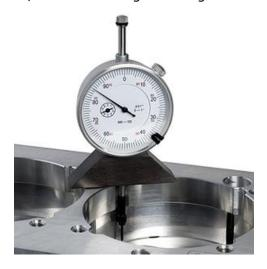
H. Replace the Cutter Head onto the Register Plate and make any groove-depth adjustments necessary, using the Depth-Adjustment Ring, to achieve the final groove depth.
