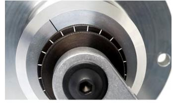
groove depth. This may be accomplished with the Depth-Adjustment Knob, or by stacking shim stock under the Depth Knob and removing a shim every two or three turns. Experiment with various techniques, to see what method works best for you. Your results may vary.
