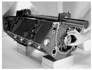
3. Gently slide the front and rear Fixture Plates onto the 2-inch Main-bearing Bar. The fixture plate with the tapped holes installs at the front of the block, with the engraved side facing out. The rear plate mounts with the "R" facing out. Slide the Angle Bracket onto the front end of the 2" Bar. Align and install three 3/8"-16 X 1" Allen Bolts. Tighten the three bolts that clamp the bracket to the 2" bar, then install and tighten the
