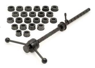
Conventional cam bearing installation tools use an expanding rubber-covered mandrel and a large hammer. This method allows the bearing to shift and potentially be driven in crooked. This can cause the camshaft to bind, leading to instant bearing failure. When installing needle type roller bearings, this method is absolutely prohibited by the bearing manufacturer, as it causes sidewall distortion, which locks the needles to the cage and prevents proper rotation.
