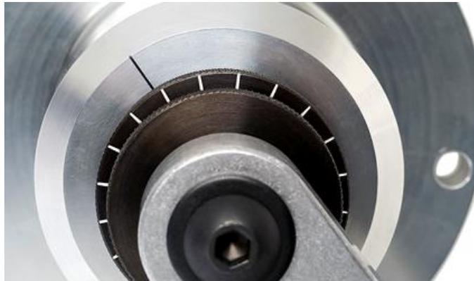
**NOTE: It is highly recommended that the desired final depth NOT be dialed-in at the start, to avoid accidentally over-cutting the groove depth for the application.**
