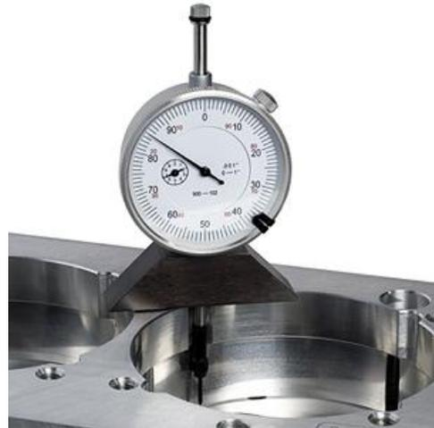
**NOTE: Uneven groove depth may be an indication that the deck surface is not even, or was not properly cleaned before installing the Register Plate. An uneven groove depth may also result if the Cutter Head is not installed securely on the Register Plate.**
